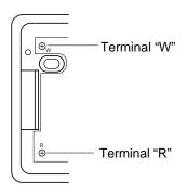
Figure 43 - Thermostat Base Terminals "W" and "R"
